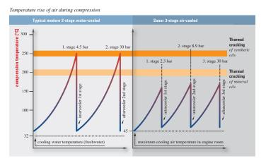
The reliable workhorse: 3-stage air-cooled compressors have been preferred for a long time by shipyards and ship-owners due to less temperature
