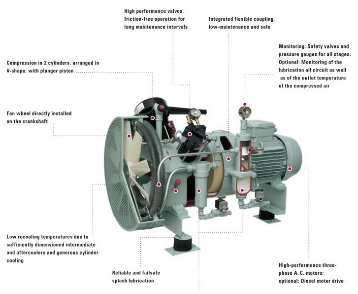
Attached separator after the 1st and the 2nd stage with automatic drainage and flexible mounting is included in the standard scope of delivery
