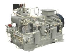
Water - cooled high pressure compressor
